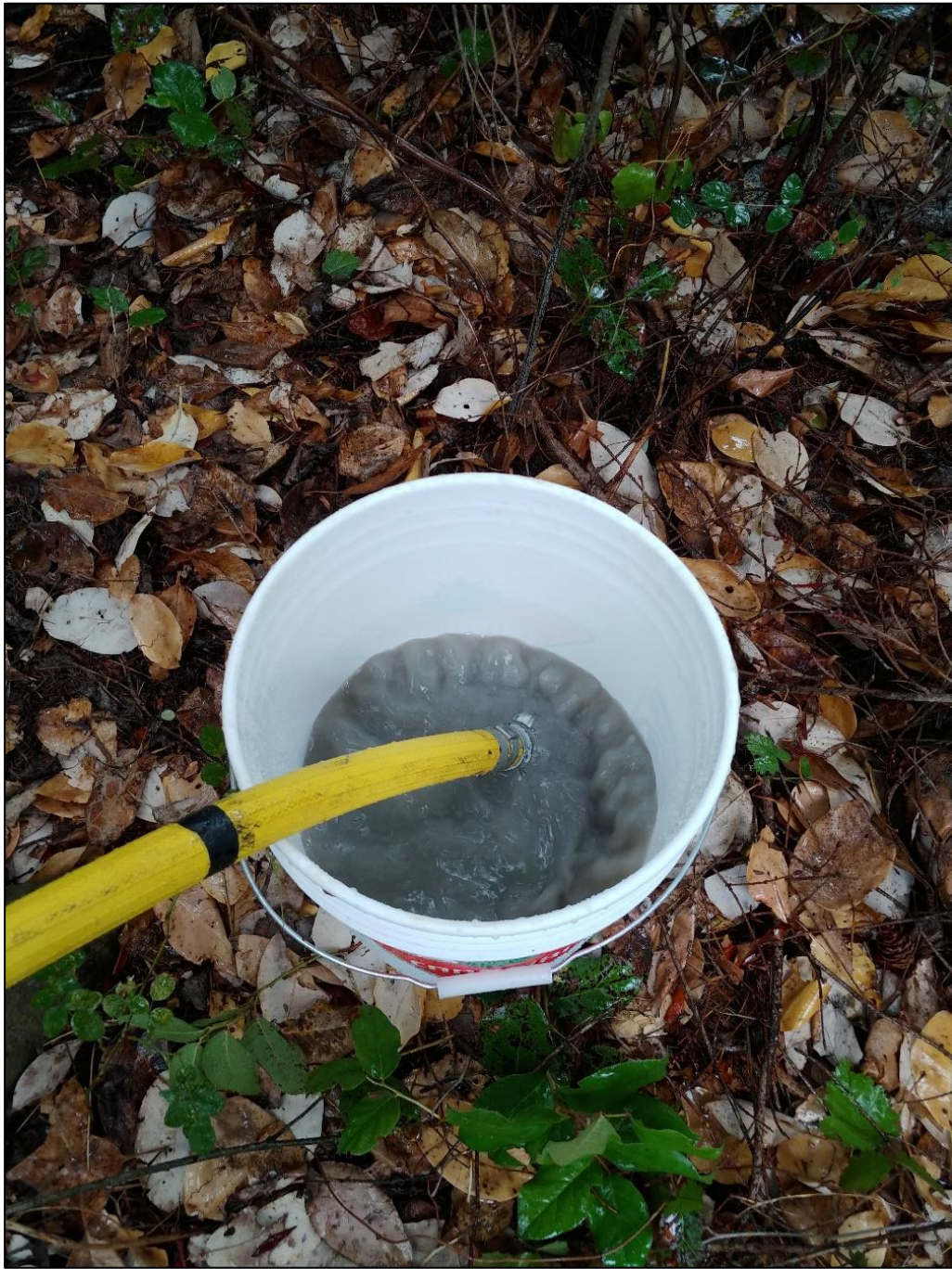
Photograph A5 (LEFT): Looking down at the 20 L pail for measuring flow rates. Photograph A6 (RIGHT): Looking down and south at the groundwater being discharging in a wooded area downslope of the well casing.
