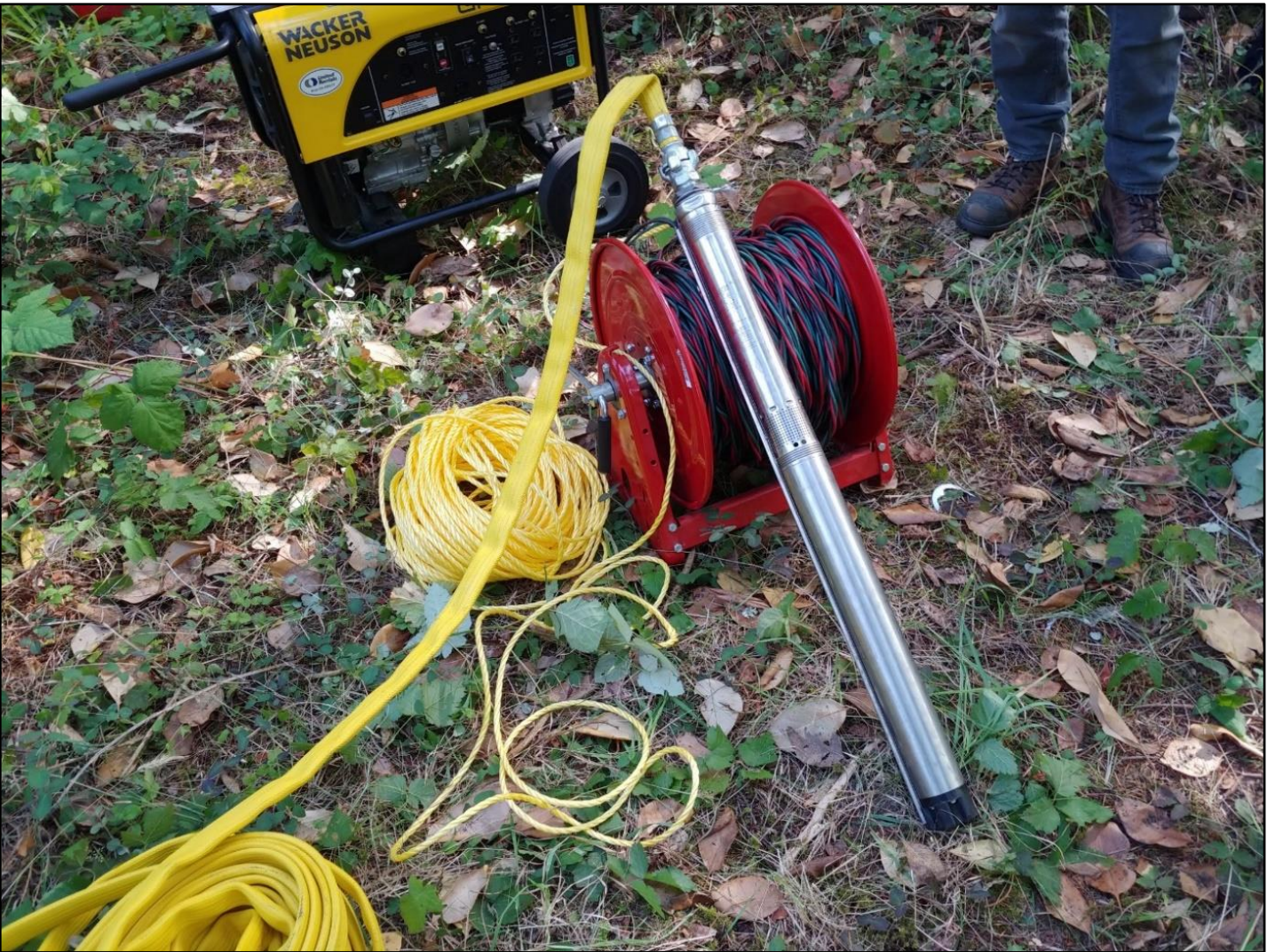
Photograph A3 (LEFT): Looking down at WIN 25234 (pumping well) with the Well Identification Number affixed to the casing. The well is properly capped. Photograph A4 (RIGHT): Looking down at the electrical submersible pump assembly with the 3” Grundfos pump and flexible hose (drop pipe)
